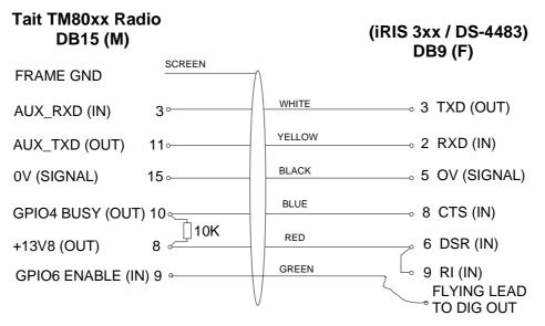
Figure 13 – Typical RS232 / Data Radio Cable
